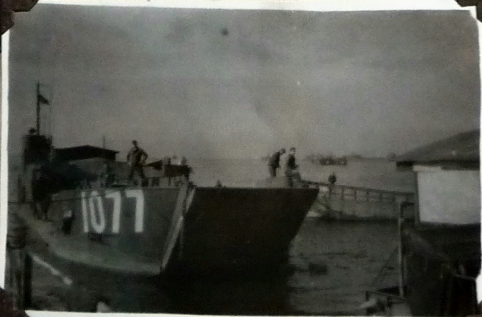
LCT coming into well-deck
