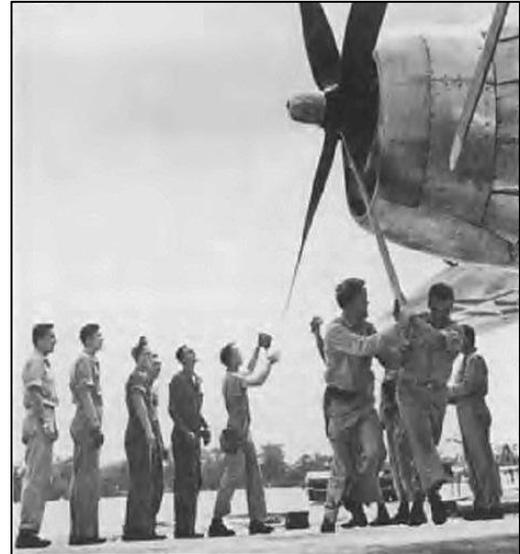
**Ground Crews “Walk the Props” of a B-29 to Remove Oil from the Engine’s Lower Cylinders Prior to Start. Source: U.S. Army**
